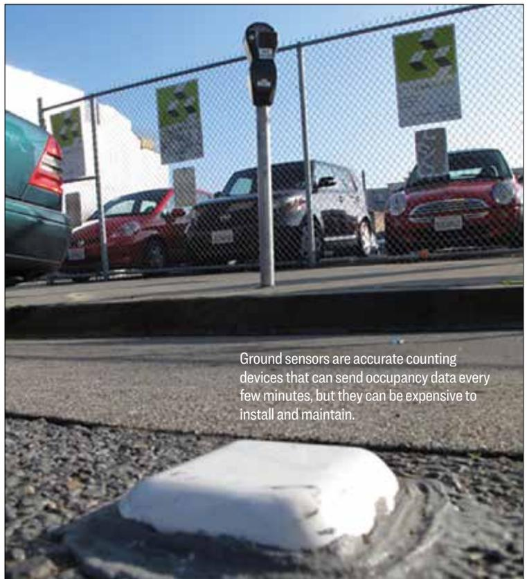
Ground sensors are accurate counting devices that can send occupancy data every few minutes, but they can be expensive to install and maintain.
