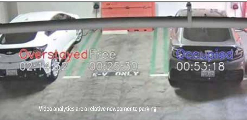
is done with cameras using still images or video clips. Technology can be limited by obstructions such as trees, sufficient lighting, and choice of mounting location. As high-end camera technology becomes cheaper to collect, the cost-per-space drops dramatically. In some cases the camera may also be able to read license plates.
